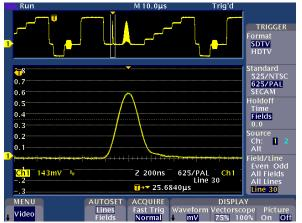
150 metres of RG59/U coaxial cable 2T Pulse waveform showing low video level and problems on the right hand side of the 2T Pulse.
