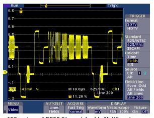
150 metres of RG59/U coaxial cable Multiburst waveform frequencies of 0.5 MHz, 1.0 MHz, 2.0 MHz, 4.0 MHz, 4.8 MHz and 5.8 MHz with the 4.8 MHz burst at -3.0 dB.
