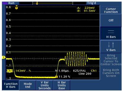
150 metres of RG59/U coaxial cable waveform showing low colour burst level of 229 mV.
