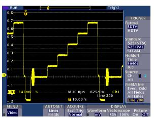
150 metres of RG59/U coaxial cable 5 Step Greyscale waveform showing low video level, rounding of the greyscale steps and horizontal sync pulse and low colour burst.
