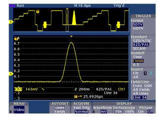
OSD 870 fibre optic system 2T Pulse waveform with an almost perfect result.
