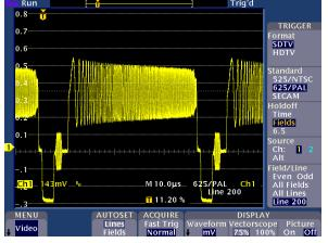
150 metres of RG59/U coaxial cable 0.5 MHz to 6 MHz Sweep waveform with no markers showing 5 MHz at -3.0 dB.
