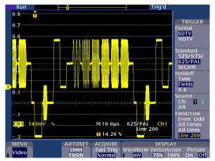
OSD 870 fibre optic system Multiburst waveform frequencies of 0.5 MHz, 1.0 MHz, 2.0 MHz, 4.0 MHz, 4.8 MHz and 5.8 MHz with the 4.8 MHz burst at +0.3 dB.
