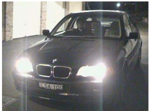
Brand Z 1/3" colour camera in the underground garage with low light levels and normal beam headlights above and full beam headlights below.
