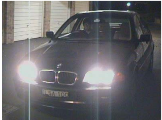
Brand Z 1/3" colour camera in the underground garage with low light levels and normal beam headlights above and full beam headlights below.
