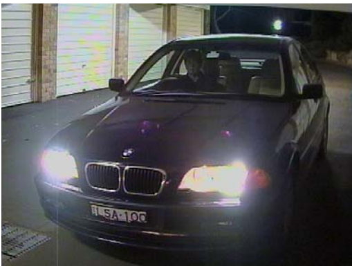
Panasonic WV-CP484E SDIII 1/3" colour camera in the underground garage with low light levels and normal beam headlights above and full beam headlights below.
