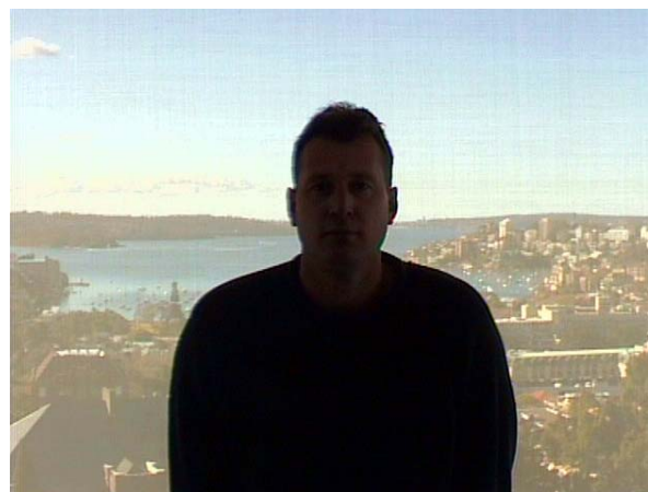
Brand Z 1/3" colour camera back light test with blind down.
