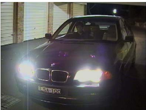
Panasonic WV-CP484E SDIII 1/3" colour camera in the underground garage with low light levels and normal beam headlights above and full beam headlights below.
