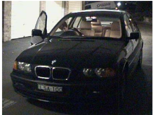
Brand Z 1/3" colour camera in the underground garage showing high random noise which is contributing to the soft image in this low light level image.
