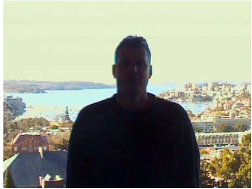
Brand Z 1/3" colour camera back light test with blind up.
